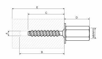
product description: M8 / M10 combined screw for quick and easy mounting of screws or threaded rods.
